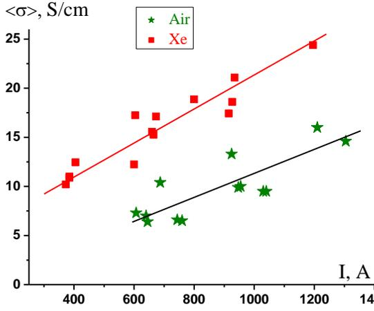
**Fig. 4.** Plasma conductivity in the near surface gas discharge in dependence on discharge current.
