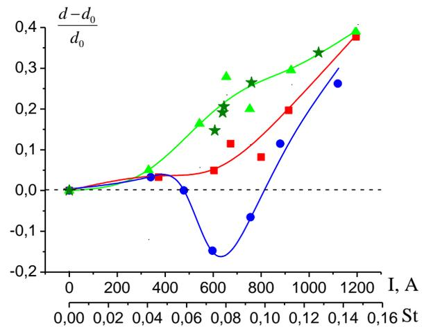
**Fig. 12.** Bow shock wave shift at EGD and MHD actions: 1 is Xe,  $B=0$  (squares); 2 is Xe,  $B=1.4T$ , Lorentz force direction is out from body (circles); 3 is Xe,  $B=1.4T$ , Lorentz force direction is up to body (triangles); 4 is Air,  $B=0$  (stars)
