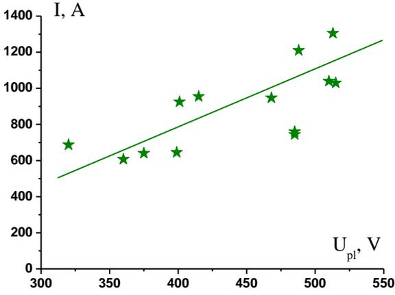
**Fig. 3.** Current-voltage curve of the near surface gas discharge in air.
