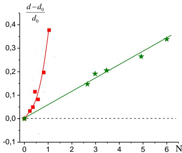
**Fig. 11.** Bow shock wave shift at EGD action: 1 is Xe,  $B=0$  (squares); 2 is Air,  $B=0$  (stars)
