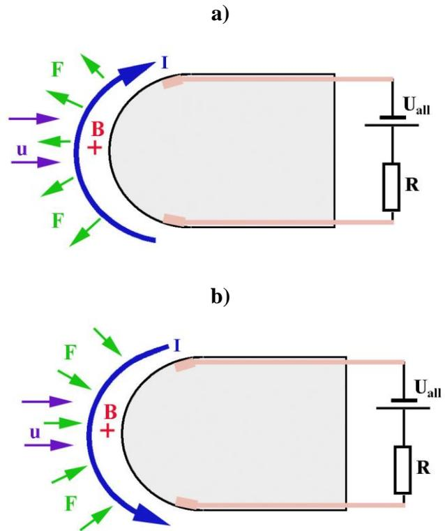
**Fig. 10.** Illustration of Lorentz force (vectors F) action at near-surface gas discharge.
