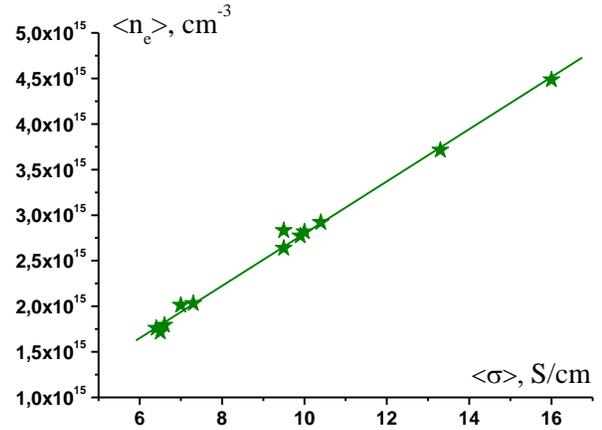
**Fig. 5.** Electron density of air in discharge in dependence on effective conductivity.
