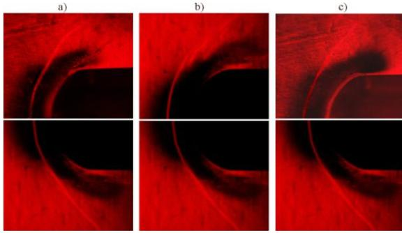
**Fig. 8.** Schlieren pictures of body streamline in air flow: top picture is obtained at near surface discharge without magnetic field; bottom picture is obtained without external action. a)  $j=3.5 \cdot 10^6 \text{ A/m}^2$ ,  $N=2.7$ , b)  $j=4.3 \cdot 10^6 \text{ A/m}^2$ ,  $N=4.9$ ; c)  $j=5.9 \cdot 10^6 \text{ A/m}^2$ ,  $N=6.0$
