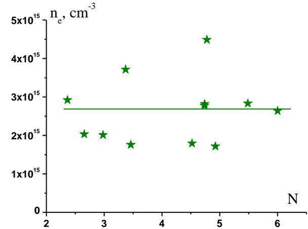
**Fig. 7.** Electron density in dependence on EGD parameter in near surface discharge.
