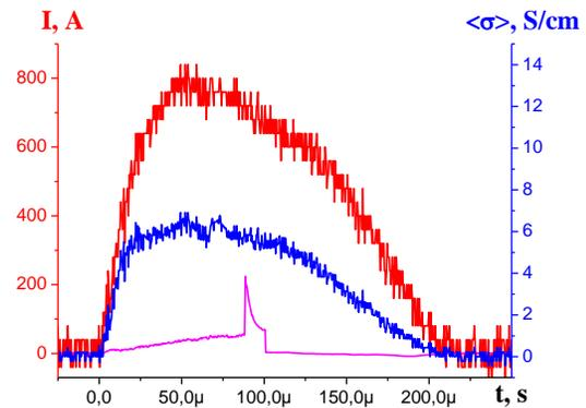
**Fig. 2.** Oscillograms of current (top curve) and integral conductivity (middle curve) of air plasma at near surface gas discharge. Bottom curve is diagnostic laser pulse.
