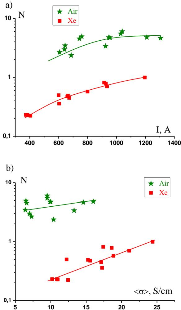
**Fig. 6.** Heating parameter in dependence on discharge current and conductivity.
