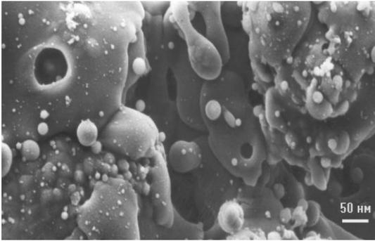
Fig.4. The structure of the deposited nanocatalysts layer after heat treatment (porosity of up to  $50 \text{ m}^2 / \text{g}$ )
