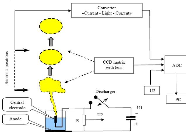
Fig.1. Principle scheme of a circuit for and “plasmoid” generation [4].
