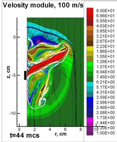
**Fig.10. Plasma Jet interaction with the cross flow at ( $\theta=135^\circ$ ).** Absolute value of a velocity distribution at the plasma jet entering the incident gas, consumption of a gas 0.2 g/s, inflowing gas pressure 0.2 atm, plasma generator power 15 kW. White area is a boundary of the plasma region.
