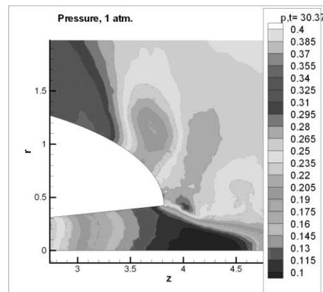
**Fig.2.** Pressure distribution at plasma jet entering the incident gas , consumption of a gas 0.2 g/s, inflowing gas pressure 0.2 atm, plasma generator power 15 kW, time  $30 \cdot 10^{-4}$  s.
