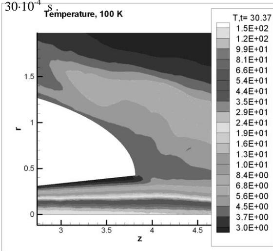
**Fig.3.** Temperature distribution at the plasma jet entering the incident gas, consumption of a gas 0.2 g/s, inflowing gas pressure 0.2 atm, plasma generator power 15 kW, time  $30 \cdot 10^{-4}$  s .
