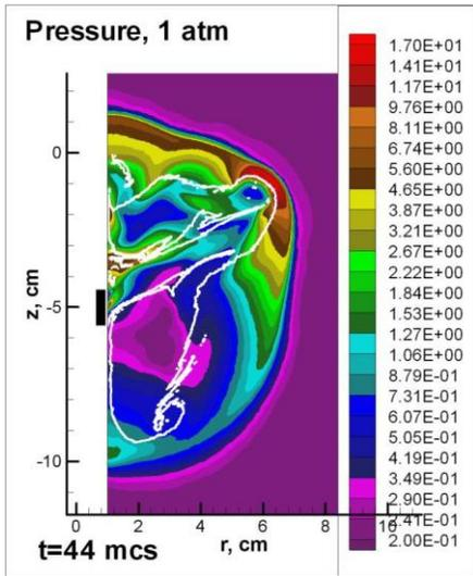
**Fig.6. Plasma Jet interaction with the cross flow at ( $\theta=135^\circ$ ).** Pressure distribution at the plasma jet entering the incident gas, consumption of a gas 0.2 g/s, inflowing gas pressure 0.2 atm, plasma generator power 15 kW. White area is a boundary of the plasma region.
