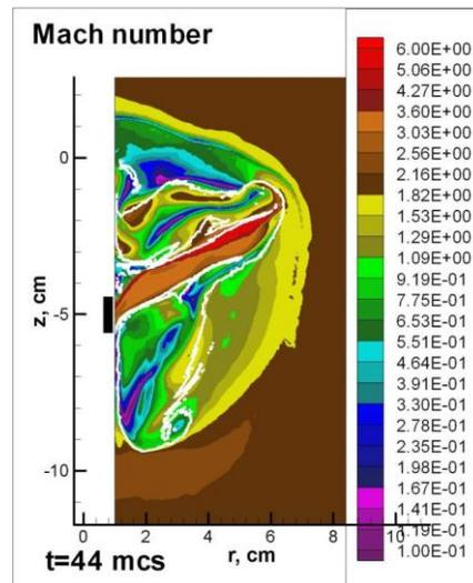
**Fig.9. Plasma Jet interaction with the cross flow at ( $\theta=135^\circ$ ).** Mach number distribution at the plasma jet entering the incident gas, consumption of a gas 0.2 g/s, inflowing gas pressure 0.2 atm, plasma generator power 15 kW. White area is a boundary of the plasma region.
