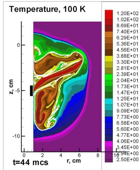
**Fig.8. Plasma Jet interaction with the cross flow at ( $\theta=135^\circ$ ).** Temperature distribution at the plasma jet entering the incident gas, consumption of a gas 0.2 g/s, inflowing gas pressure 0.2 atm, plasma generator power 15 kW. White area is a boundary of the plasma region.
