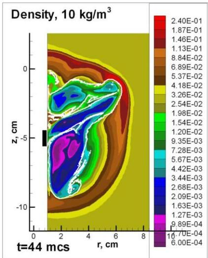
**Fig.7. Plasma Jet interaction with the cross flow at ( $\theta=135^\circ$ ).** Density distribution at the plasma jet entering the incident gas, consumption of a gas 0.2 g/s, inflowing gas pressure 0.2 atm, plasma generator power 15 kW. White area is a boundary of the plasma region.
