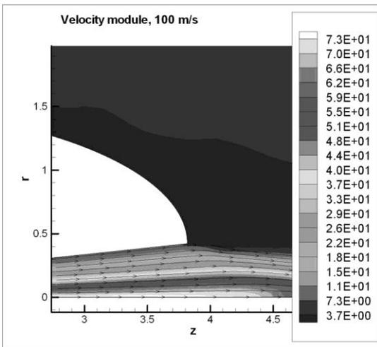
**Fig.5.** An absolute value of the velocity distribution at the plasma jet entering the incident gas, consumption of a gas 0.2 g/s, inflowing gas pressure 0.2 atm, plasma generator power 15 kW, time  $30 \cdot 10^{-4}$  s .
