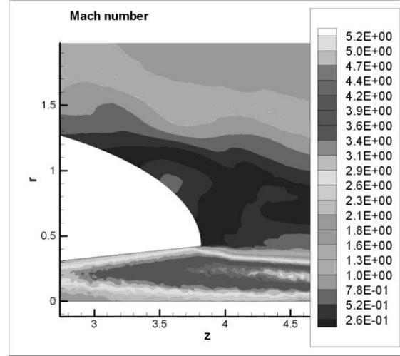
**Fig.4** Mach number distribution at the divergent plasma jet entering incident gas , consumption of a gas 0.2 g/s, inflowing gas pressure 0.2 atm, plasma generator power 15 kW, time  $-30 \cdot 10^{-4}$  s .
